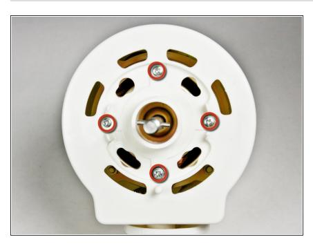
Remove the front motor housing by removing 4 screws.
