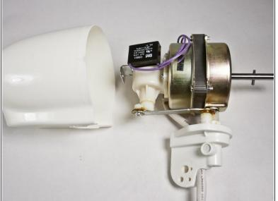
The main motor housing can be taken off by removing a single screw at the back of the upper assembly.
