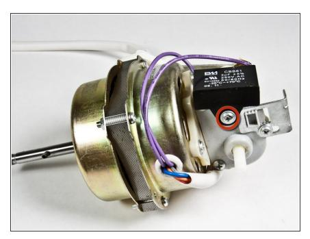
There is a capacitor attached to the oscillator by a single screw. Once the screw is removed the capacitor should come off easily.
