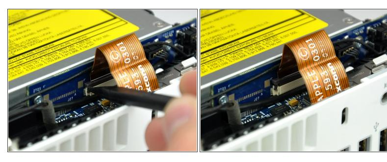
Use the tip of a spudger to slightly lift the left side of the ZIF cable lock up from its socket.
