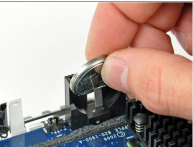
Push the PRAM battery toward the center of the logic board and pull it up out of its holder. You'll
