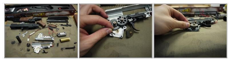
• Reinstall the gears and trigger assembly, making sure that all of the shims are in their original position, and that the anti-reversal latch is seated properly with the spring in place.
