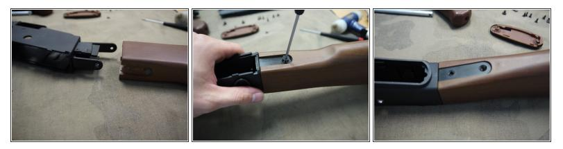
• Slide the stock back on the receiver and reinstall the three screws that hold it in place.
