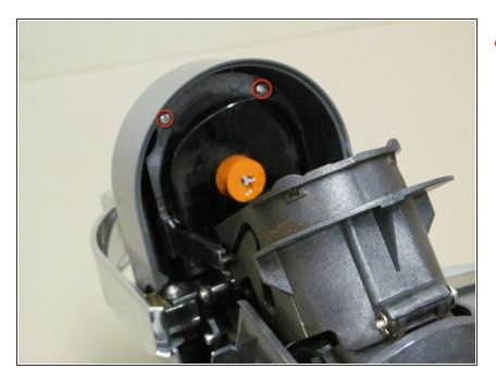
Remove the two 12mm Phillips screws using a Phillips #0 screwdriver.
