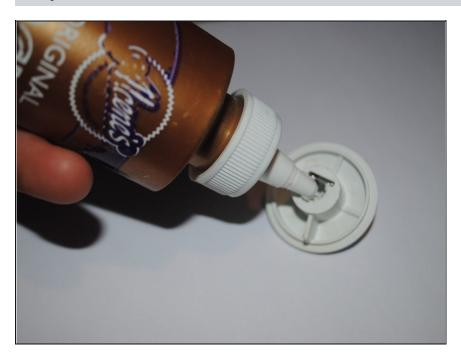
Apply polyurethane glue to the inside of the metal tab.
