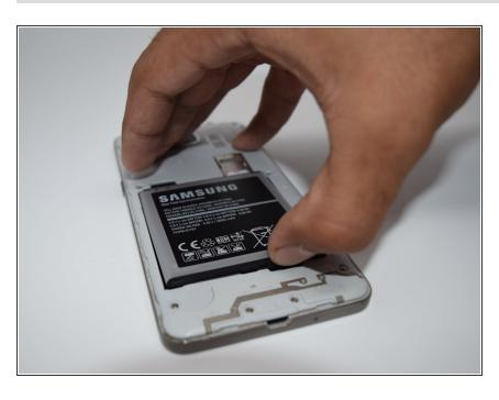
To remove the battery, lift up on the thumb tab located on the bottom right corner of battery bay.
