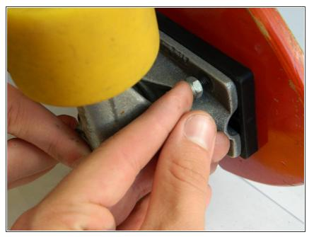
• Hand tighten the nut hardware onto all four bolts.
