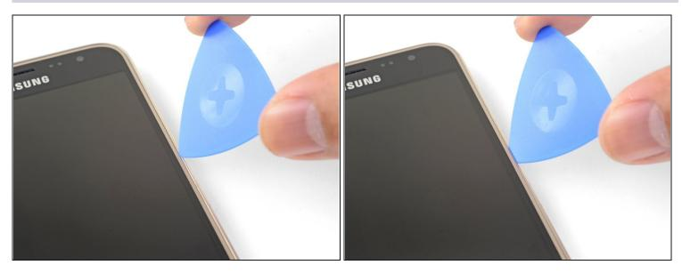
• Firmly press an opening pick into the right edge seam of the phone, until the point slides in between the frame and the display glass.
