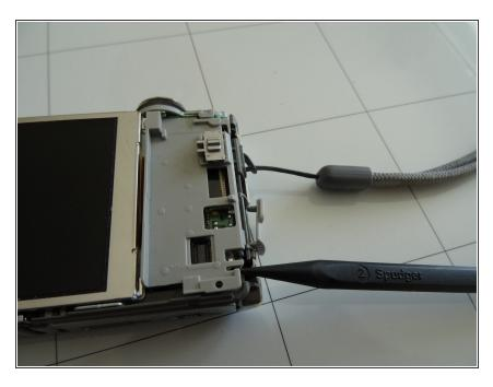
• Under the keyboard board you will find a gray plastic molding. This part is just jammed and with a bit of patience you can remove it with a spudger. Make sure that none of the sensitive detents break off. Start prying at the bottom.
