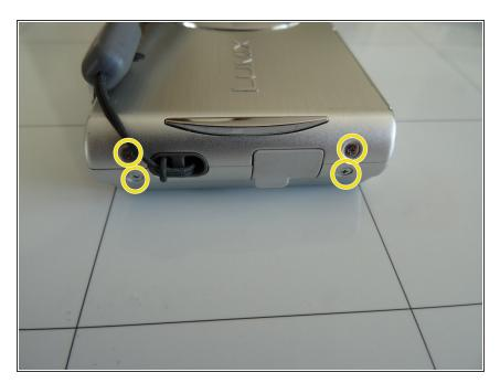
Remove the four 3.3 mm Phillips screws from the left side
