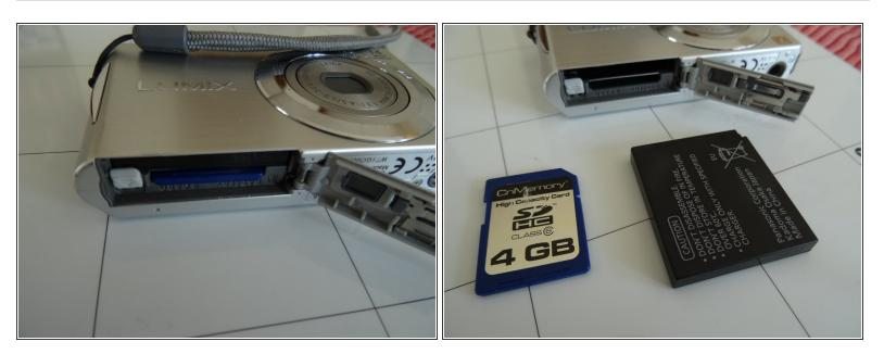
Open the battery compartment cover and remove the battery and the memory card,
