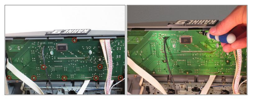
• Remove the screws that are holding the circuit board in place.
