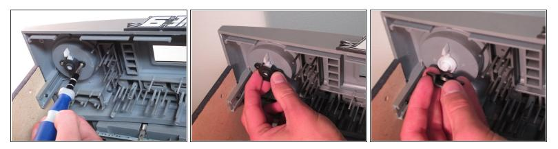
• Remove the screws and the black piece that are holding the volume control knob in place.
