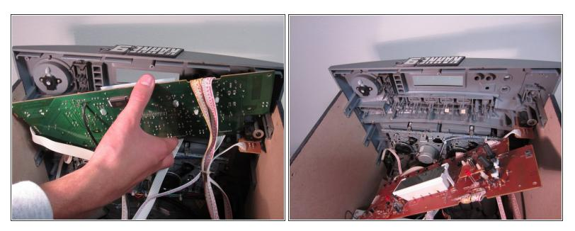
• Pull the circuit board out to reveal the inside of the display.
