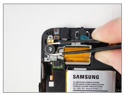
• Pull the vibrator up and out of the socket to remove.
