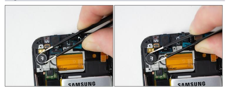
• Grip the vibrator motor with a pair of blunt nose tweezers and wiggle the motor to loosen it from the adhesive.
