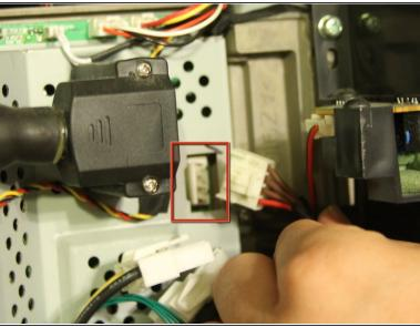
• Disconnect the lamp ballast power connection and the light engine power connection by pressing down the tab and pulling out the connection.
