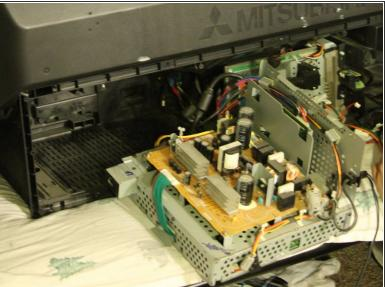
Pull out the protective case holding the power supply and input/output boards.
