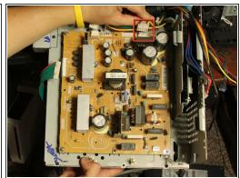
Unplug the power connections on the power supply board by pressing down the tabs on the connections and gently pulling the connections away from the board.
