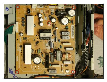
Remove the five 10 mm silver, coarse threaded Phillips #0 screws securing the power supply board to the case.
