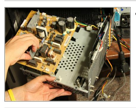
Remove the power supply board from its protective case by pulling it straight up and away from the case.
