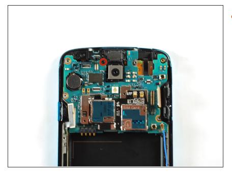
Remove the single 2.4 mm Phillips #00 screw from the motherboard assembly.
