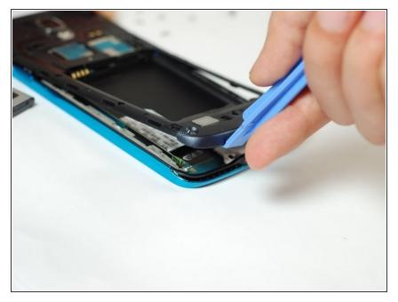
• Use the plastic opening tool to pry around the entire edge of the midframe now to release it from the front case.
