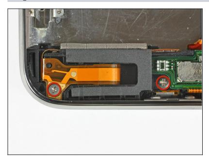
Phillips screws securing the upper logic board to the rear panel.
