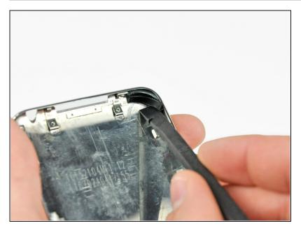
Use the flat end of a spudger to pry the protective rubber grommet from the bottom left hand corner of the rear panel.
