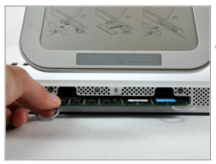
Slide the RAM chip straight out of its socket.
