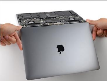
Keep the main body secured against the table and open the screen all the way.
