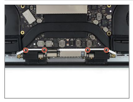
Remove the four 3.9 mm T3 Torx screws securing the two display cable cover springs.
