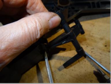
That's the trickiest part: you have to lever this lever out of its camp. To do this you drive with a screwdriver between the lever and the carrier and press it really very strong outwards. Now he grabs out - hopefully!
