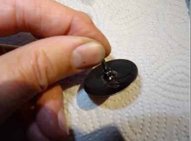
With a 6mm Allen key (or the key that comes with the machine), the brewing sieve can be unscrewed. It strongly determines the aroma, if it is dirty the coffee tastes bad.
