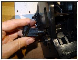
Through the hole on the opposite side of the fixing screw can be solved. The inlet is plugged in and held by a latch, which you have to push away.
