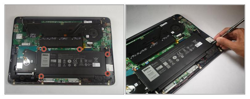
• Remove the five 5.0 mm-long Philips #0 screws that connect the battery to the case.
