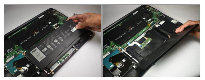
• Lift the battery out of the case.
