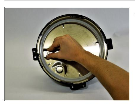
Pull the plastic washer off the bobber valve and allow the bobber valve to fall out
