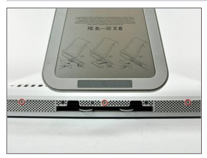
Remove the three T8 Torx screws securing the front bezel to the rear case along the lower edge of the iMac.
