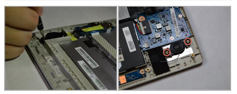
Unscrew the two 3mm screws with the PH1 screw head on each speaker found on the corner's away from the hinges.
