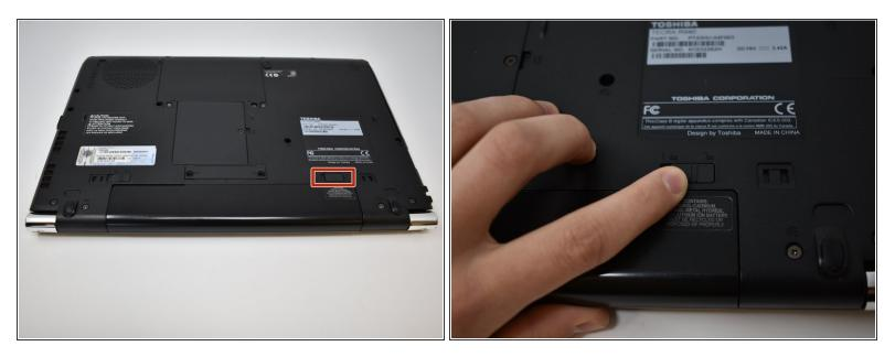
• Slide lock 1, located on the right side, to the unlocked position.
