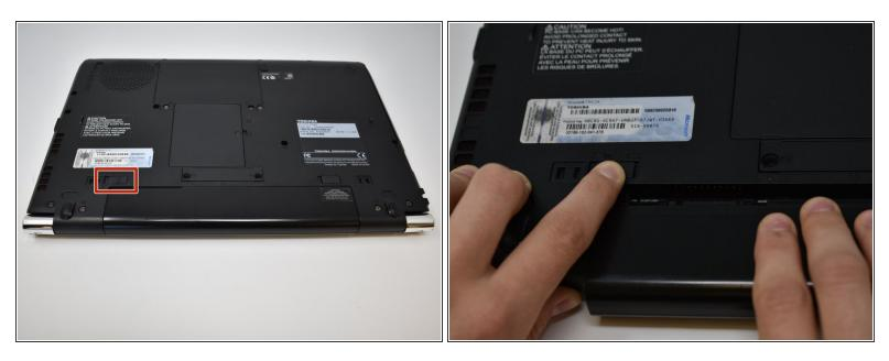
While holding lock 2 (left side) in the unlocked position, pull out the battery pack.
