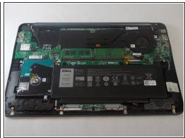
Remove the plastic heat spreader that covers the RAM sticks.
