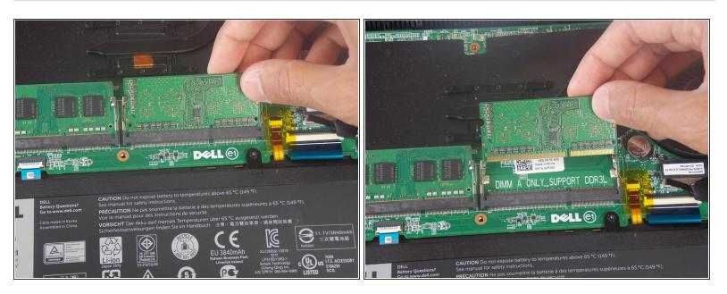
Pull the RAM stick in a straight line out of the socket.
