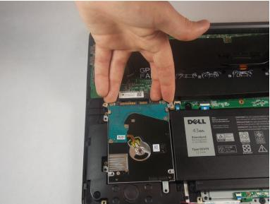
Disconnect the hard drive from the motherboard by placing your fingers at the back, and pulling forward towards the front of the chassis.
