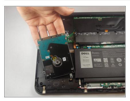
Lift the hard drive out of the chassis.
