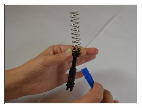
Using a tool such as a spudger, gradually maneuver spring off of telescopic piston.
