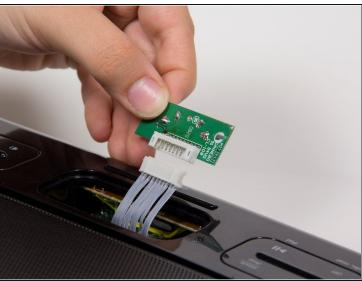
Carefully pry apart the bundle of white wires connected at the junction with the plastic opening tool.
