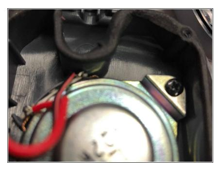
Unscrew the 2 screws holding the driver unit to dismantle the driver.
