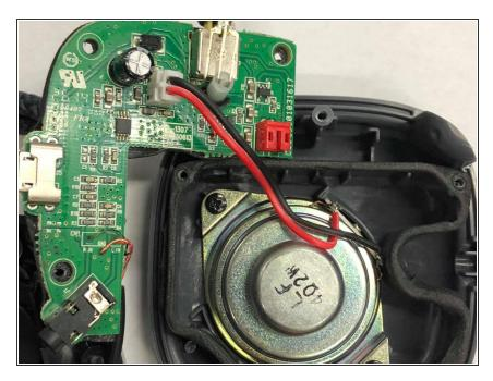
Unplug the wore from the driver and battery, be careful as not the pull the wire, instead, pull the plug to avoid breaking the wire.
