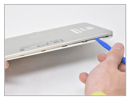
Slide the opening tool along the seam between the back panel and the screen panel, prying the panels apart as you move around the edges.
