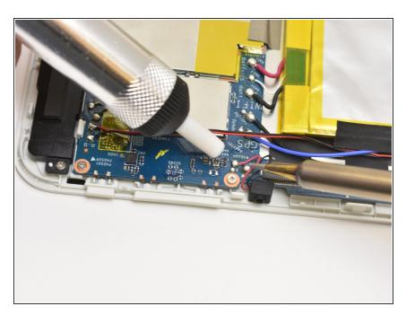
Desolder the microphone wires from the motherboard.
