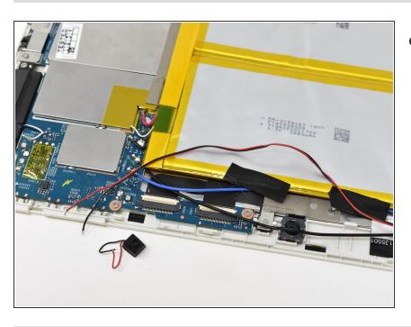
Separate the microphone from the rest of the device.
