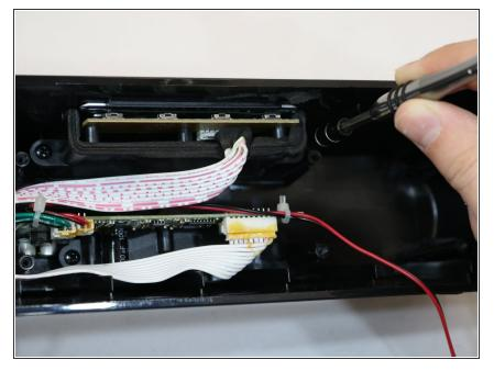
Unscrew upper panel two 10 mm screws spinning a size PH2 screwdriver in a counterclockwise motion.
