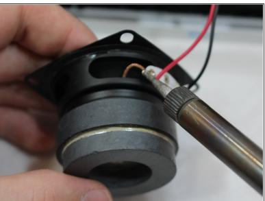
Remove green (left) and red (right) wired connection to speaker bulb using a soldering station.
