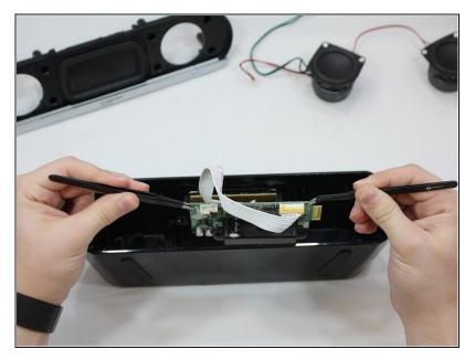
Pull motherboard out of slot using the angled tweezers and blunt nose tweezers on each side.
