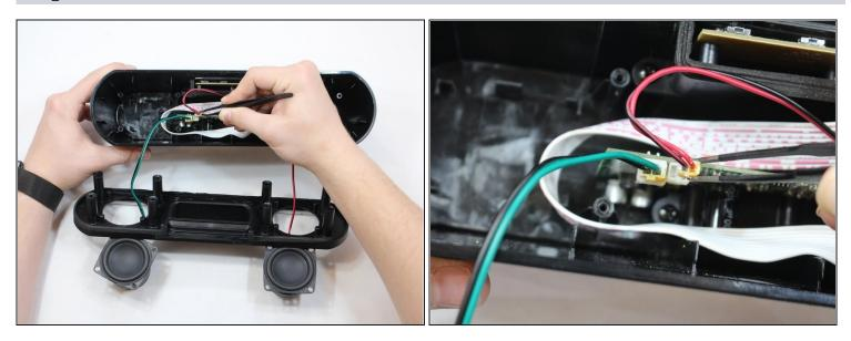
Pull wires out of ports using blunt nose tweezers.
