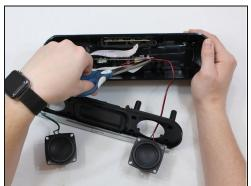
• Cut zip-ties wrapped around red and green wires using scissors or pliers.
