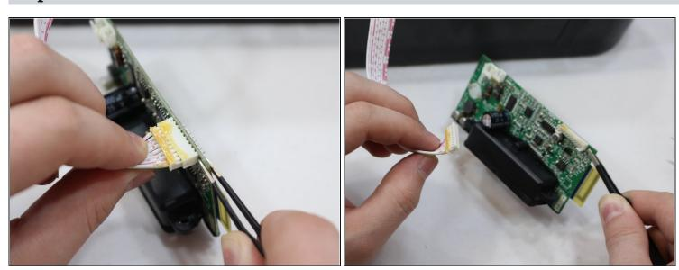
• Remove motherboard from white wire strip by pulling the two apart using blunt nose tweezers on one side and fingers on wire strip plug.
