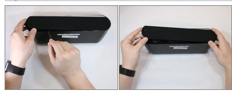
Remove front panel by forcefully placing the flat edge of the spudger in between panel and plastic. Angle spudger and use fingers to pry panel off. You may need to use extra force.
