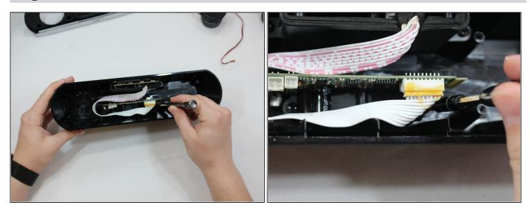
• Unscrew two 10 mm screws below connecting motherboard to speaker system by spinning a Phillips PH2 bit screwdriver in a counterclockwise motion.
