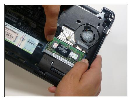
Push out the two plastic prongs on either side of the RAM.
