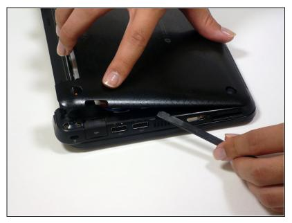
i If the back case does not separate from the netbook easily, use the spudger to pry off the back case by the edge near the battery compartment, and work your way to the sides. The case will then pivot along the front edge.
