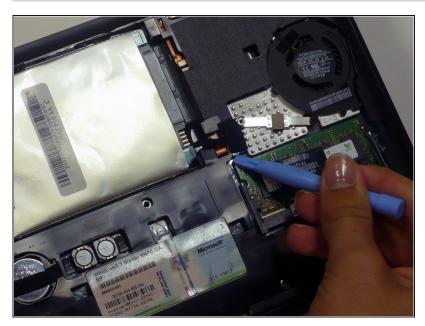
Use a plastic opening tool to carefully disconnect the hard drive connector found above the RAM slot.
