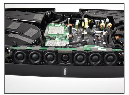
Prop the removed main speaker array up on top of the main circuit board.
