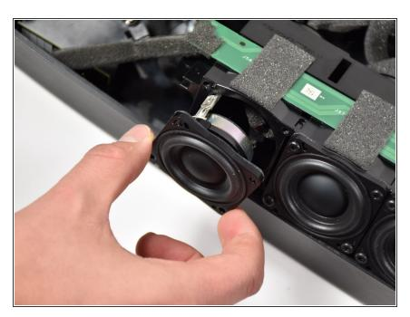
Remove the damaged speaker from the array socket, by grasping the speaker with one hand, the array with your other and pulling outward.
