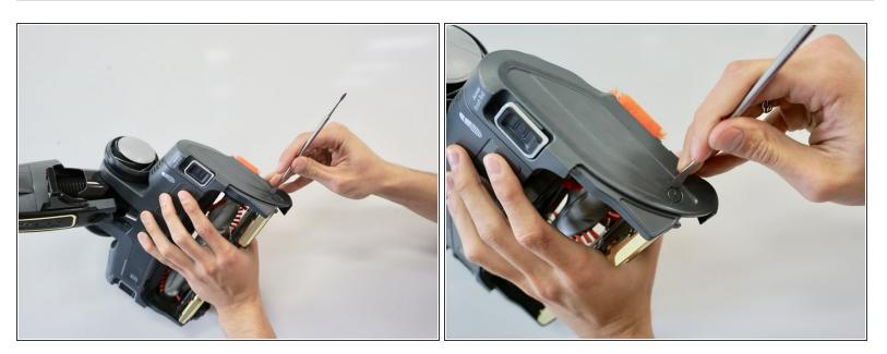
• Remove the plastic screw covering using a metal spudger by pushing the sharp side into the crevice and prying the cover out.
