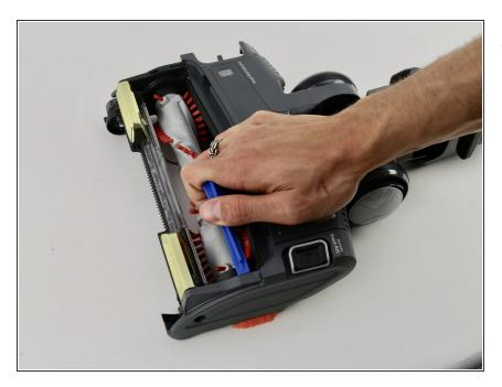
• Use the iFixit Opening Tool to pry the side of the vacuum open.
