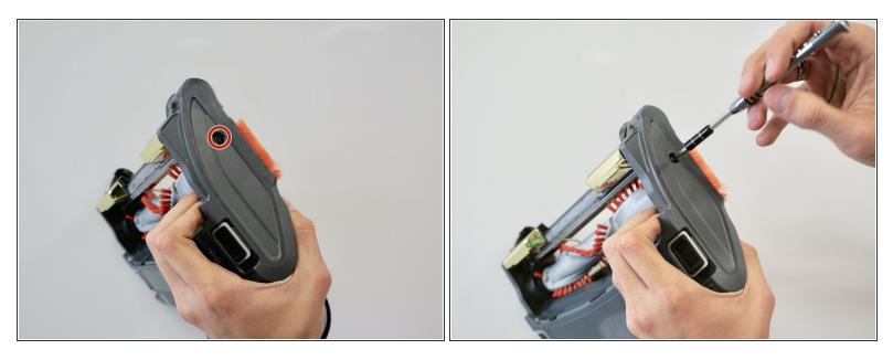
• Turn the T10 Security Torx screwdriver counterclockwise to remove the 15mm screw.
