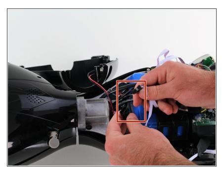
Unplug the lights from the battery by pulling gently on both sides of the black connector attached to the white wires.
