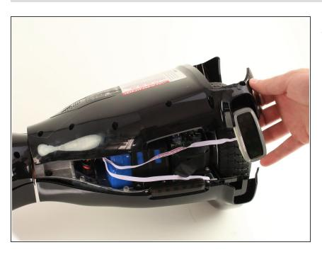
Remove the vertical light from the shell by using your hands to pull it free from the surrounding shell.
