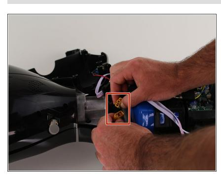
Unplug the battery by pulling gently on both sides of the orange connector.
