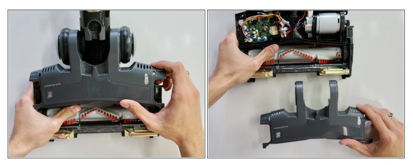
• Using the plastic spudger, pry the back seam of the top component to pop it off the vacuum.
