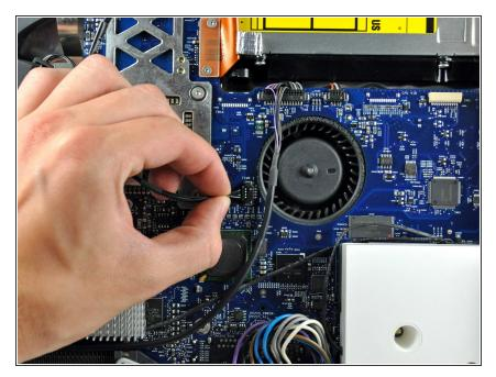
Disconnect the optical drive thermal sensor by pulling its cable toward the left edge of your iMac.
