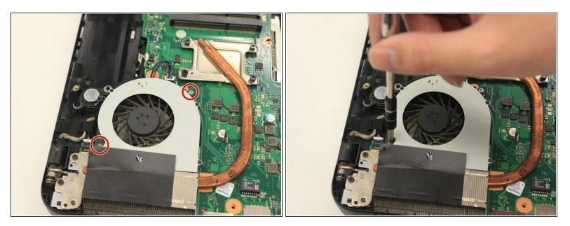
• Remove the 2 screws holding the fan in place.
