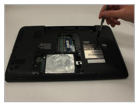
Using the PH1 screwdriver, remove the remaining screws from the back casing of the laptop.
