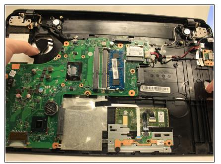
• The screws holding the keyboard in place have already been removed along with the back panel, so just push the keyboard out of the laptop by pushing your fingers through the holes under the fan and CD drive.
