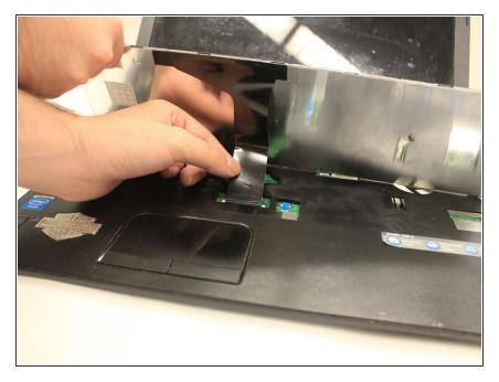
Once the keyboard is hanging out of the laptop, separate it from the device by pulling out the tab connecting the keyboard to the motherboard.
