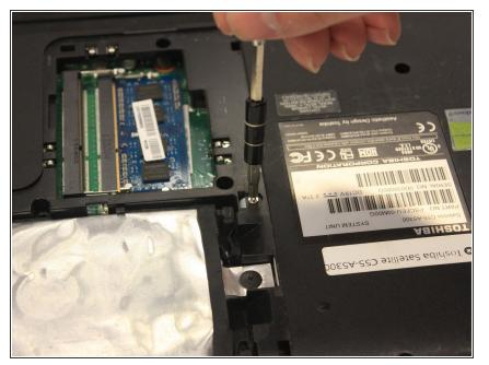
Remove the screw to the top right of the hard drive using the PH1 screwdriver.
