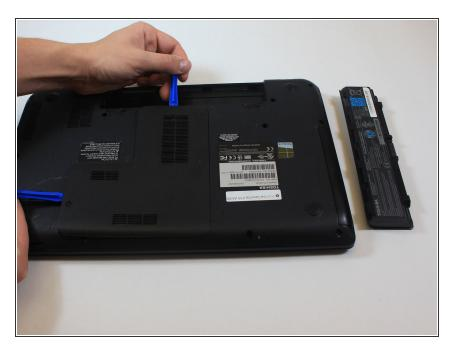
• Use the plastic opening tools to remove the panel.
