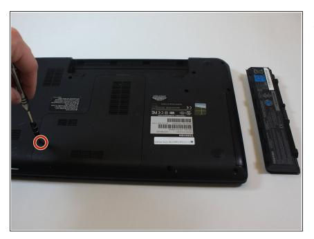
Unscrew the screw on the back panel of the laptop covering the hard drive.
