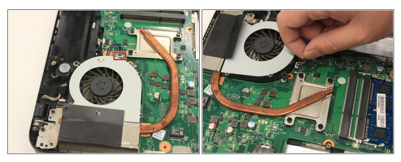
• Detach the multi-colored wire connecting the fan to the motherboard and pull the fan out.
