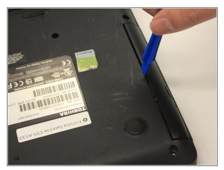
Use the plastic opening tool to wedge between the CD Drive and the laptop casing and gently pull it out.
