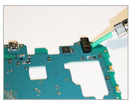
Use the soldering tool to remove the audio jack. To reassemble your device, follow these instructions in reverse order.
