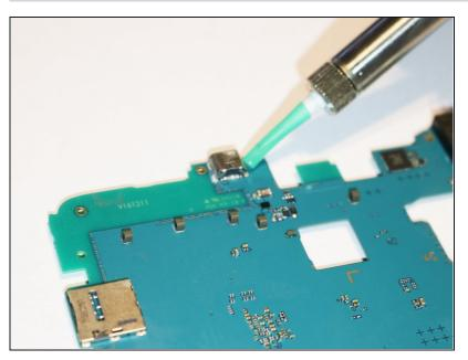
• Use the soldering tool to remove the charging port.
