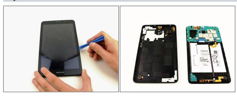
• Use the iFixit Opening Tool to pry off the back case, moving the tool around the screen.
