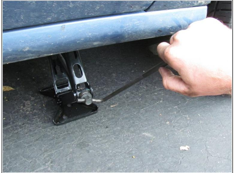
**⚠ Do not go under the car unless the car is support by a jack stand.**
