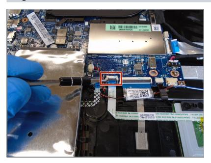
Before removing touchpad you will have to disconnect it from the circuit board using a nylon spudger.
