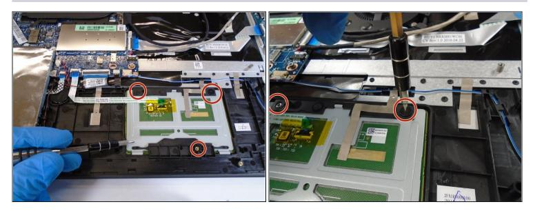
• Remove all the screws holding the touchpad down.
