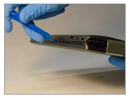
Pop off the back panel using a plastic opening tool once all screws are removed.
