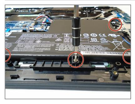
Once the panel is fully removed, begin to unscrew the battery.
