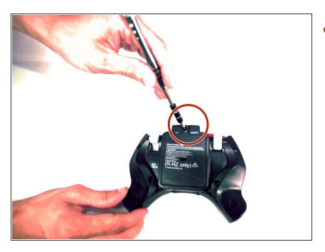
• Use a JIS #0 screwdriver to unscrew the single battery cover screw.
