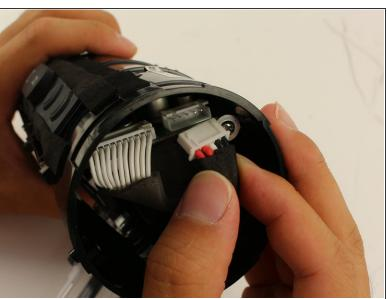
Pull gently to disconnect the bundled cable connector in the side of the speaker. This action will separate the battery from the motherboard.
