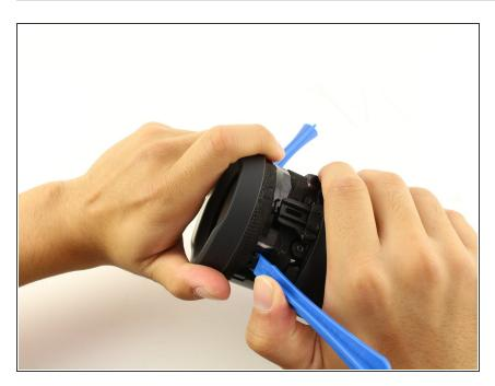
Twist and pull open the passive radiator. The left radiator twists off clockwise; the right counterclockwise.
