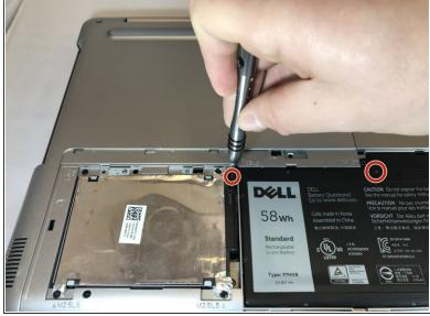
Remove the two black PH1 6mm screws that anchor the battery.
