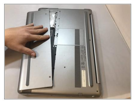
Apply pressure with your fingertips on top of the cover and drag toward the front of the laptop. This will make the plate slide off exposing the hard drive.
