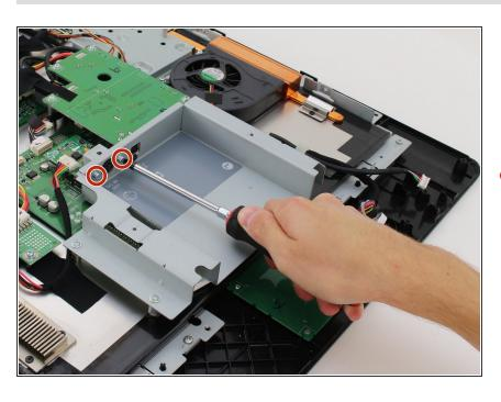
Remove the two 7.8mm Phillips #2 screws from the right back panel connected to the power port by
