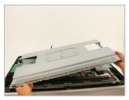
Remove the back metal plate by lifting up along one edge, then lifting the plate off and away from the device.
