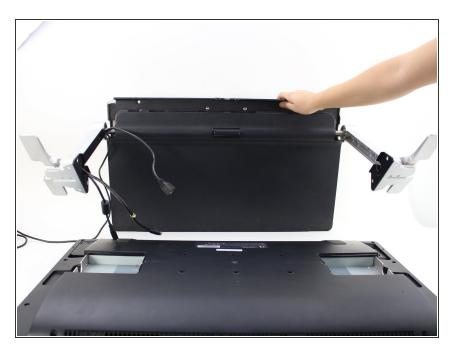
Lift the stand up and away from the rest of the device so the legs separate from the mounting plate.
