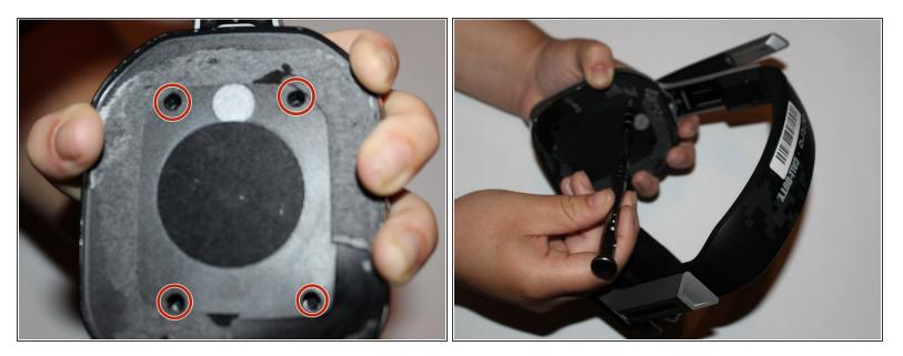
• Remove the four 7mm screws with a Phillips #1 screwdriver.
