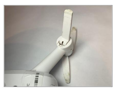
Turn the drone over so the propellers are facing down. Pull the leg up so the leg is pointed up towards the ceiling.
