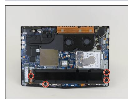
• Remove the four 4 mm Phillips #00 screws securing the battery.
