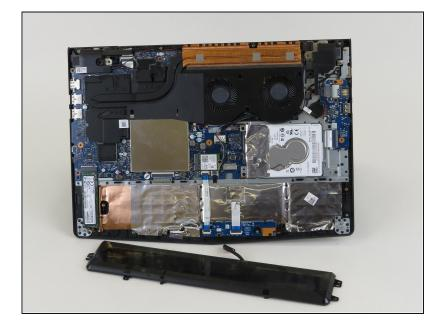
• Lift the battery up and out of the chassis.
