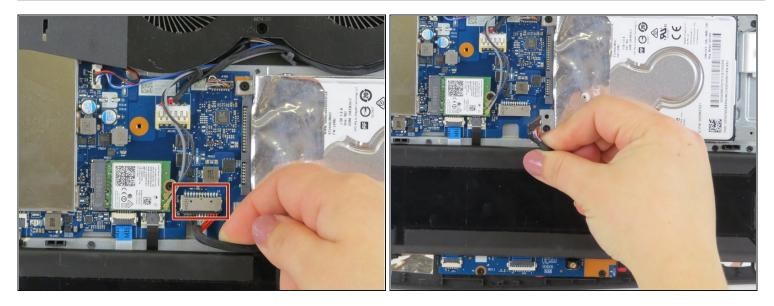
Disconnect the battery connector by pulling the battery cable directly out of its port, toward the battery.
